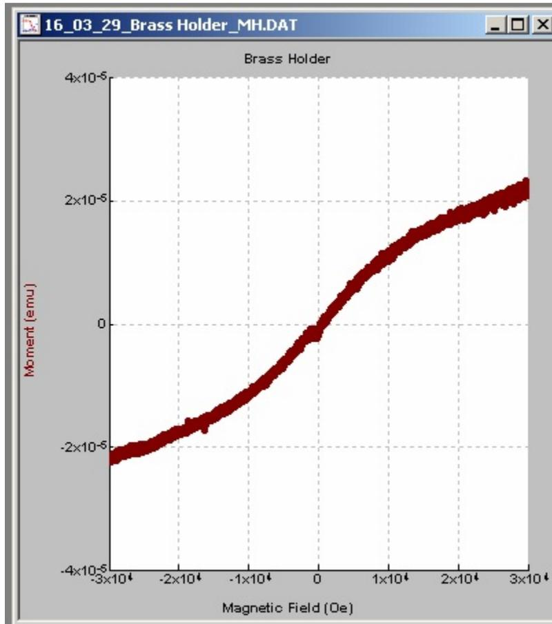
Figure 2. Moment vs. field for the brass holder without sample. Always determine the sample holder background before performing measurements.
