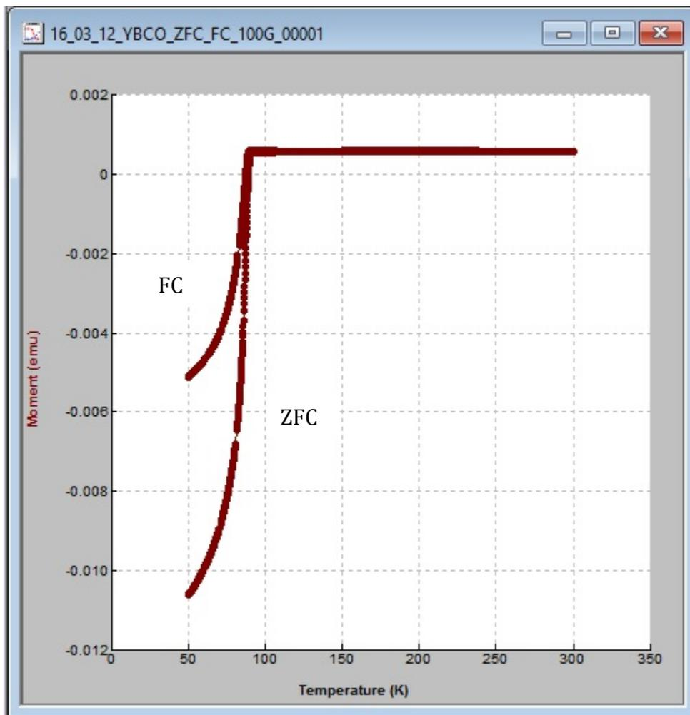
Figure 11. Moment vs. temperature data demonstrating the Meissner effect. The upper lower magnitude region is FCC, demonstrating flux trapping, while the more negative magnitude plot region is ZFC.
