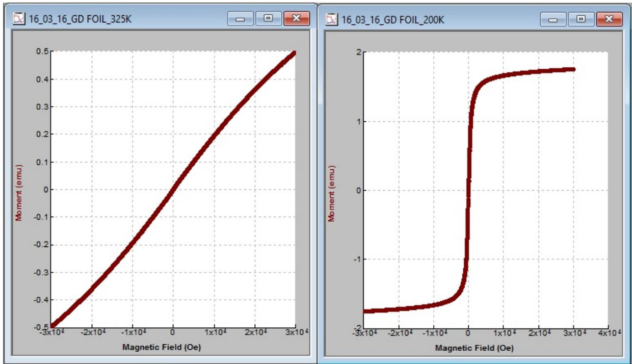
Figure 6. (left) Gd foil measured at 325 K, above the Curie temperature; (right) Gd. Foil measured at 200 K, below the Curie temperature.
