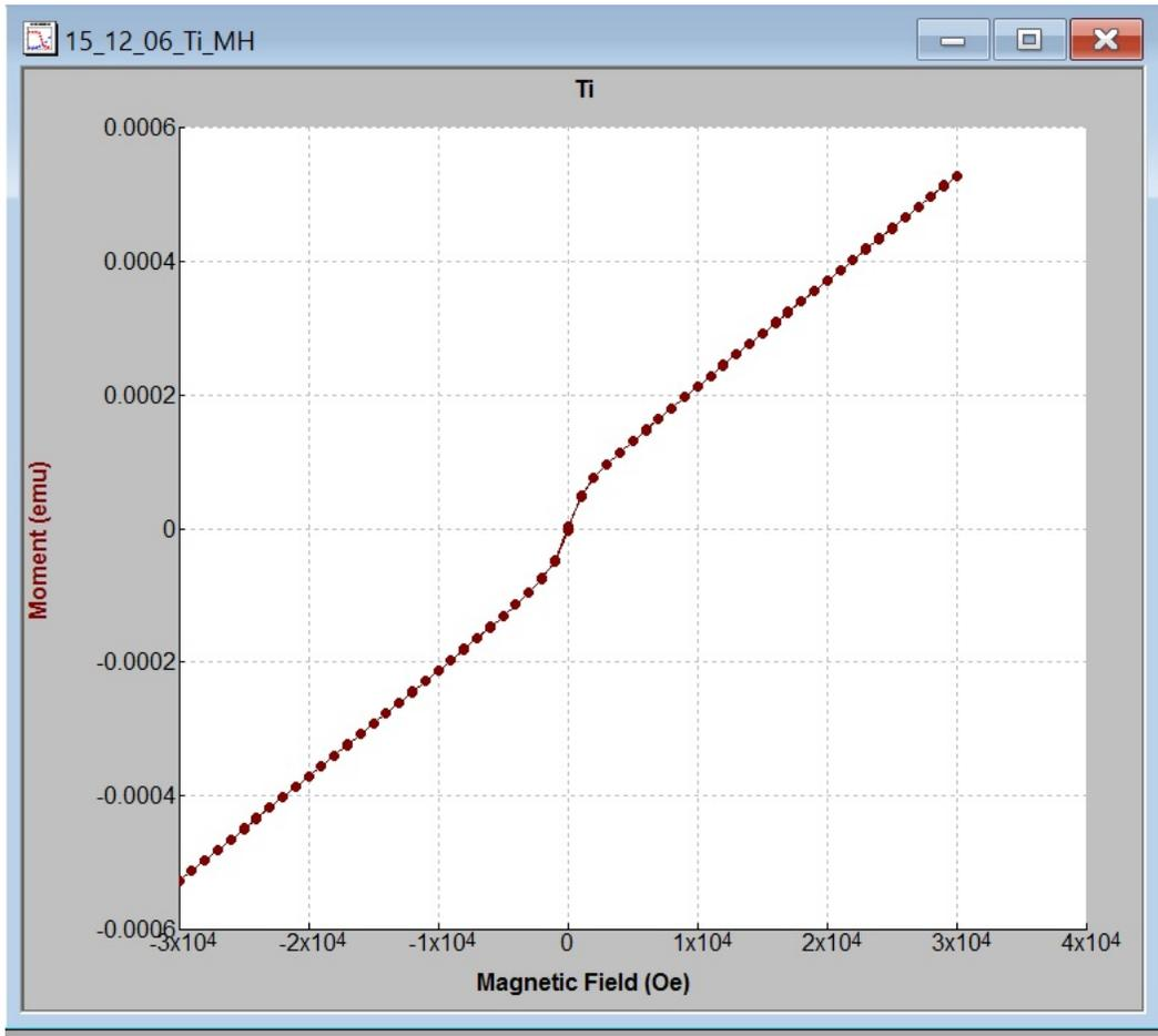
Figure 5. Moment vs. field for Ti foil at 300 K showing paramagnetic behavior, with a low field kink that may be due to sample impurities.
