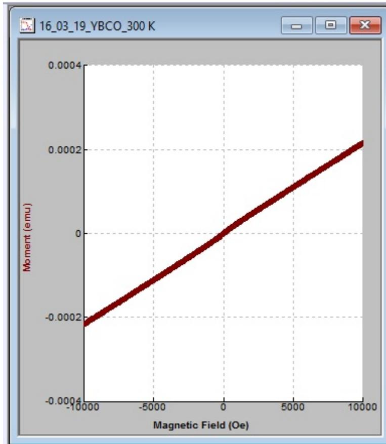
Figure 12. YBCO in the normal state possesses paramagnetic moment vs. field behavior.
