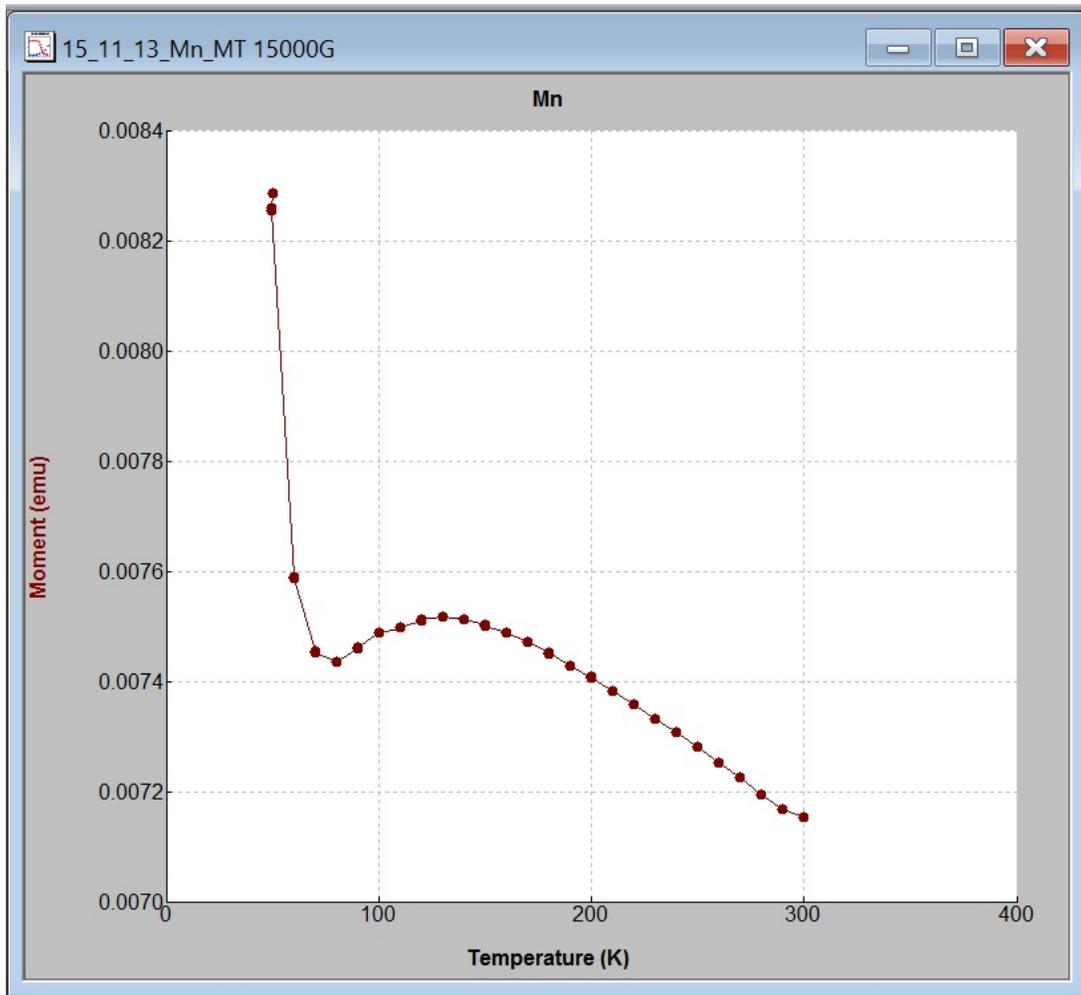
Figure 9. The magnetic moment vs. temperature for Mn with oxidation on its surface performed at 1.5 T. The low temperature region indicates the presence of an impurity.
