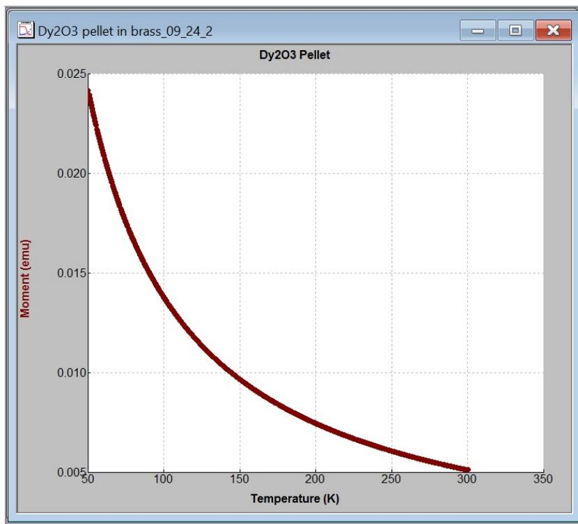
Figure 3. Measurement of magnetic moment vs. temperature using  $H = 1000$  Oe for  $\text{Dy}_2\text{O}_3$  sample.
