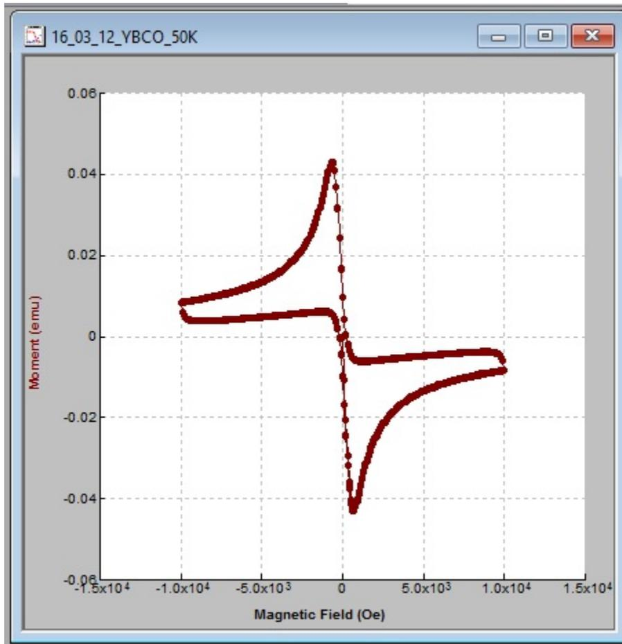
Figure 13. Moment vs. field data below  $T_C$  at 50 K showing hysteresis in the mixed state in a Type II superconductor.
