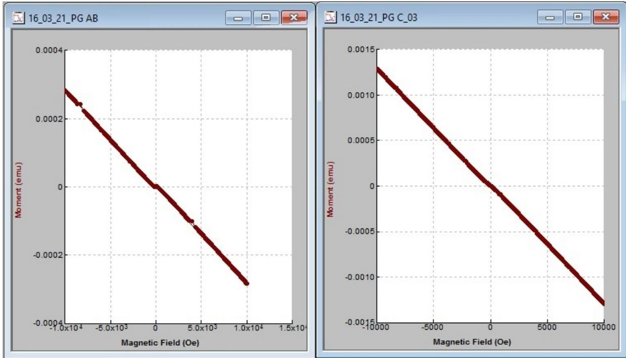
Figure 10. Moment vs. H for a sample of pyrolytic graphite, oriented with the field perpendicular to the c-axis (left) and parallel to the c-axis (right), performed at 300 K. Note the stronger magnetic moment in the c-axis.
