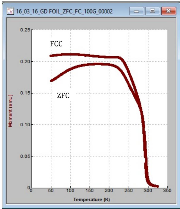
Figure 7. Moment vs. temperature data for the Gd foil with the ZFC being the down-turned plot and the FCC being the upper plot. Gaps in the high temperature data may be due to the re-centering of the sample holder during measurement.
